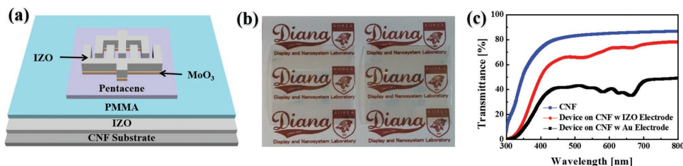
Figure 1. a) Bottom-gate/top-contact OPT device structure on a CNF substrate. b) A photograph of the OPTs above the DIANA Lab logo. c) Optical transmittance spectra of the CNF substrate and of the devices on CNF substrates with IZO and Au S/D electrodes.
