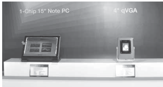
< 4> Oxide TFT-LCD 1-chip 38.1 cm Note PC( ), printable oxide TFT-LCD 10.2 cm qVGA( )
