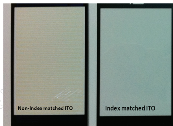
Fig. 6. Visibility of ITO patterns: non-index-matched ITO (left) and index-matched ITO (right).
