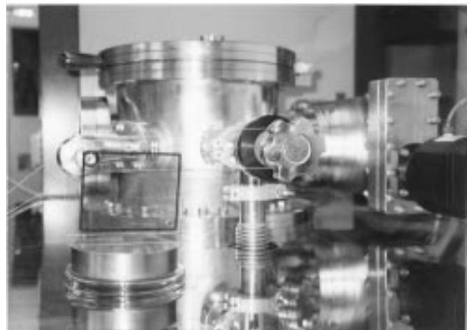
Figure 7. Hermetic sealing test of an FED panel with an exhausting hole sealed by glass-to-glass bonding.
