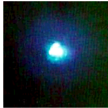
Fig. 9. The emission pattern V_g = 55V , I_a = 2.0\mu A
